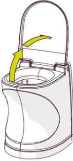
Lift up the lid and the seat. The red light flashes and the green light is illuminated. The exhaust fan will start automatically.
