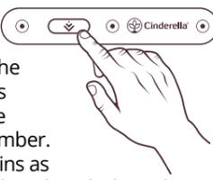
Push the "Start" button to drop the bowl liner and its contents into the incineration chamber. Incineration begins as soon as the hatch is closed. The toilet is now ready for the next user.
